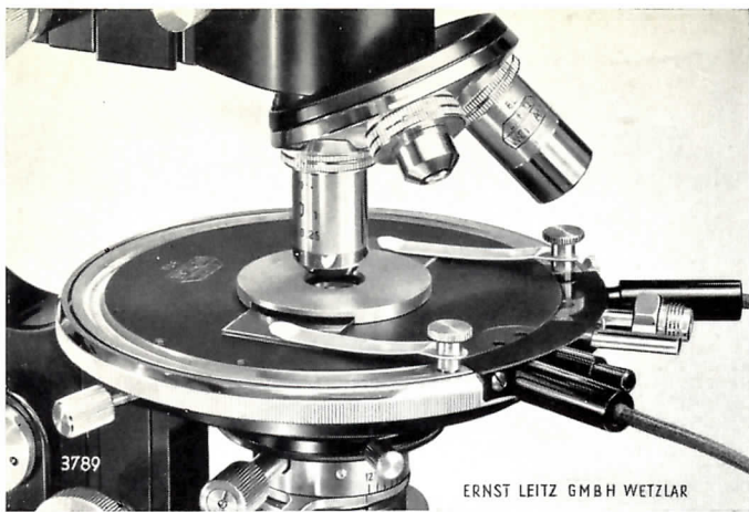
Heating stage with temperature stabilizing chamber
