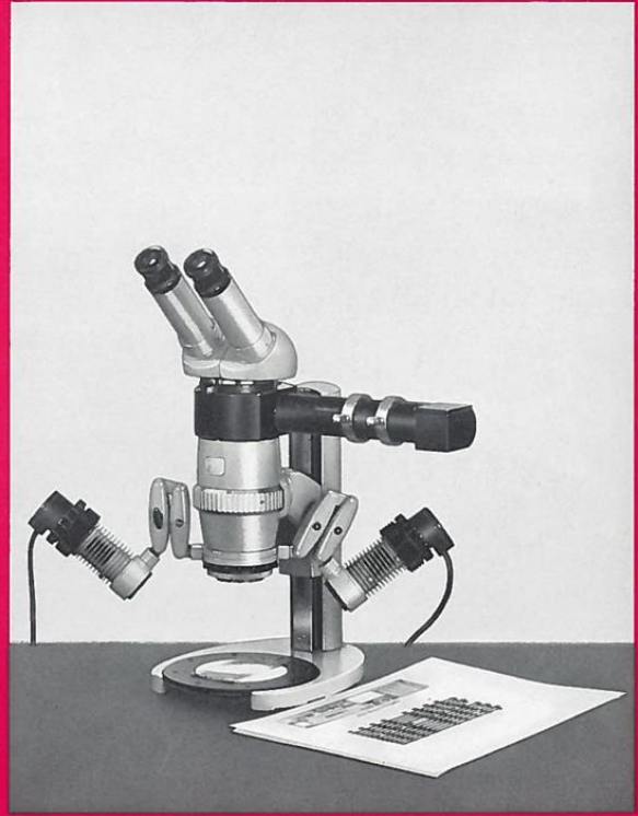
The camera lucida used on a Stereomicroscope IV for comparing an etched printed-circuit board with the original drawing.
